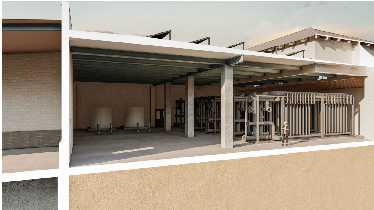
Figure 6-5. Conceptual Reverse Osmosis System Cross Section
