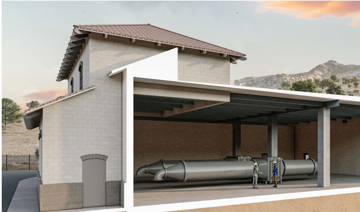
Figure 7-2. Ultraviolet Advanced Oxidation Process Cross Section
