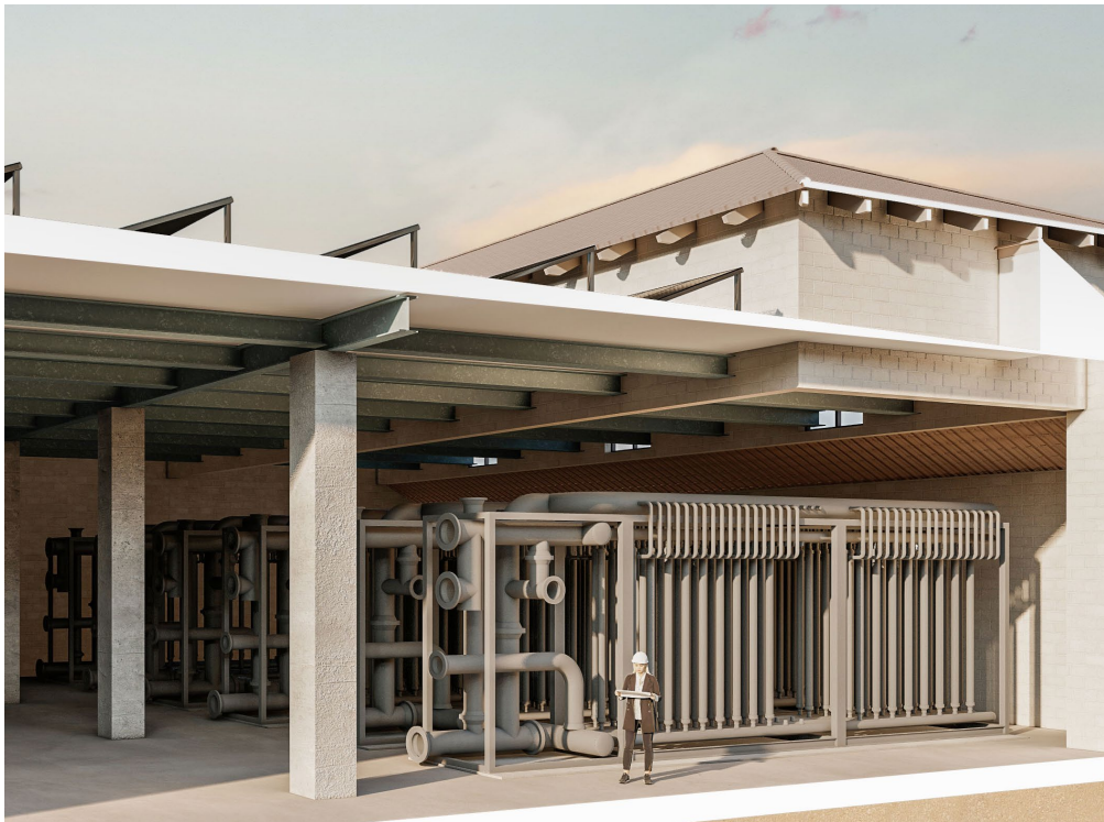
Figure 5-3. Conceptual Membrane Filtration Section
